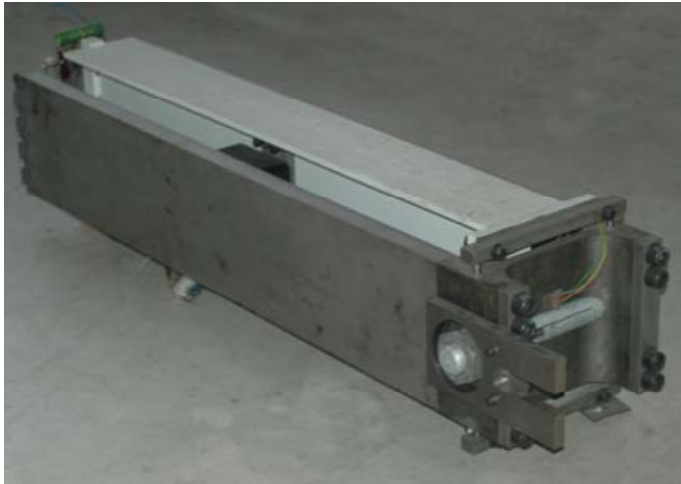
Figure 2-15: left: testing machine for fatigue test under pure bending (Pat.-No. 10 04 258), right: flange segment connection for fatigue test und combined loading; Berger & Schaumann (2008)
