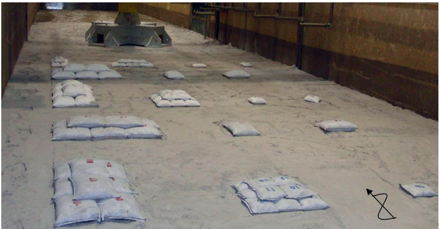
Figure 4-6: Arrangement of sand-filled geotextile containers (before test).
