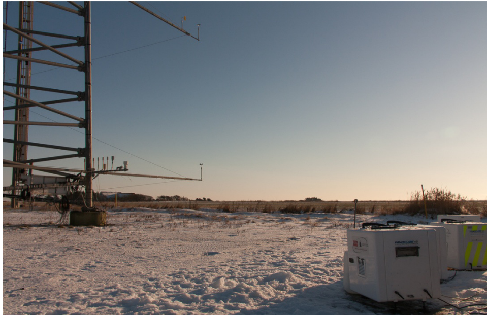
Figure 5-11 Lidars under calibration at the Høvsøre Test Station.
