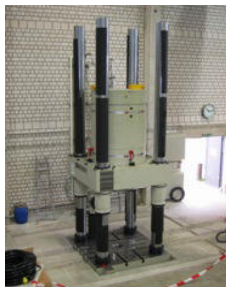
Figure 2-12: Test facilities at LUH, left: “SincoTec” Magnetic resonance max. force 400 kN, right: “Instron” Servo-hydraulic, max. force 10 MN
